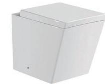
GD-HT920B Back to wall toilet Size: 555x355x395mm S-trap: 100mm Roughing-in P-trap: 180mm Roughing-in
