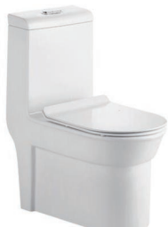
Cody Four hole Eddy One- Piece toilet Size: 690x380x750mm S-trap: 300/400mm Roughing-in
