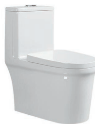
GD-1280 Siphonic One-Piece toilet Size: 700x380x750mm S-trap: 300/400mm Roughing-in
