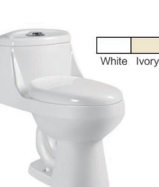
GD-0335A Siphonic One-Piece toilet Size: 730x350x630mm S-trap: 250/300/400mm Roughing-in
