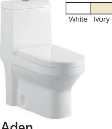
Aden Siphonic & Washdown One-Piece toilet Size: 710x370x790mm Siphonis: S-trap: 250/300/400mm Roughing-in Washdown: P-trap: 180mm Roughing-in S-trap:100/250/300mm Roughing-in
