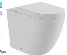
GD-HT9034B Back to wall toilet Size: 550x365x400mm S-trap: 120/150mm Roughing-in P-trap: 180mm Roughing-in
