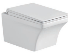
Baykal Washdown Wall-hung toilet Size: 530x360x330mm P-trap: 180mm Roughing-in
