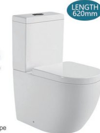
GD-T003B-R Washdown two-piece toilet Size: 620x375x820mm S-trap: 220/250mm Roughing-in P-trap: 180mm Roughing-in
