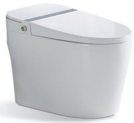
HP-2201C Smart One-piece toilet Size: 680x390x490mm Material : Ceramic Bowl & ABS Cover S-trap : 300 / 400mm P-trap : 180mm Heating moed : Non-Cistern Rapid Heating Type Rated voltage : 110V-220V Color : White
