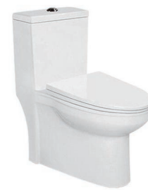
Calanda Washdown One-piece toilet Size: 710x385x755mm S-trap: 250mm Roughing-in P-trap: 180mm Roughing-in
