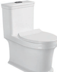
Cole Four hole Eddy One- Piece toilet Size: 700x380x720mm S-trap: 300/400mm Roughing-in
