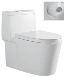
GD-5517 Siphonic One-Piece toilet Size: 710x410x640mm S-trap: 300/400mm Roughing-in
