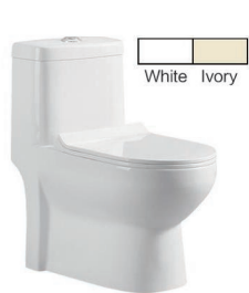
GD-1443 Siphonic & Washdown One-Piece toilet Size: 640x380x700mm S-trap: 250/300mm Roughing-in
