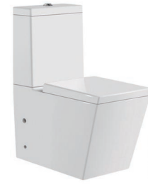
GD-T001B Washdown Two-piece toilet Size: 685x360x830mm S-trap: 250mm Roughing-in P-trap: 180mm Roughing-in
