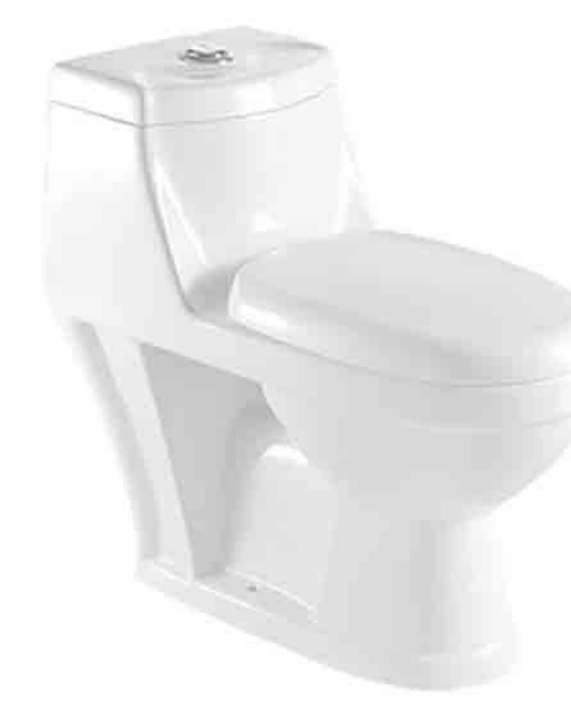
GD-2081 Washdown One-Piece Toilet Size:710x370x660mm S-trap:100/200/250/300mm roughing-in P-trap:180mm roughing-in
