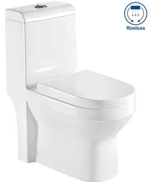
ADEN Washdown/Siphonic One-Piece Toilet Size:695x366x805mm S-trap:250/300mm roughing-in P-trap:180mm roughing-in
