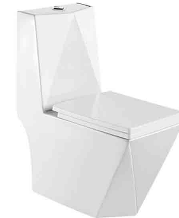
GD-20389 Washdown/Siphonic One-Piece Toilet Size:680x370x795mm S-trap:250/300mm roughing-in P-trap:180mm roughing-in
